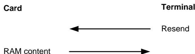
215 In this example, whether the TOE actually dumps the memory contents depends on the proper initialisation of I/O buffer pointer and length. The memory shown in the example might contain residual secret data, for example a recently calculated DES session key. Therefore this attack may allow an attacker to retrieve secret data from the TOE.
