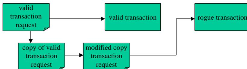
220 The picture shows a situation where the attacker copies a valid transaction request, modifies it and sends a second request using the same (or slightly modified) versions of
